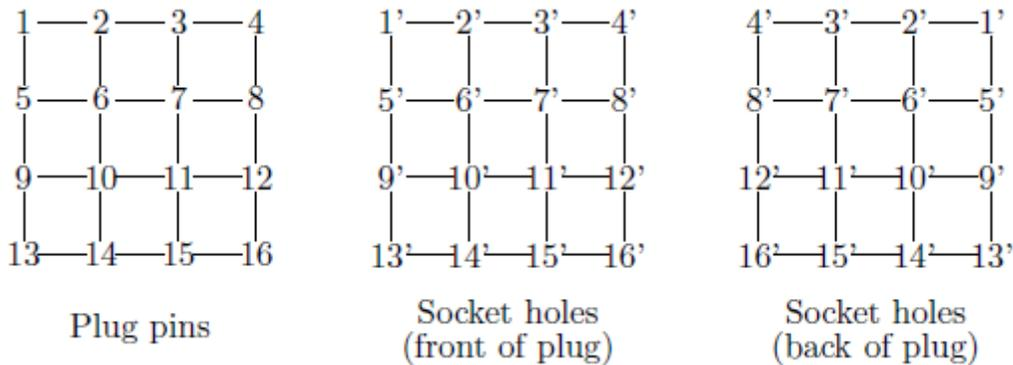
Clearly pin 1 can be connected only to holes 1', 4', 13', or 16' (depending on how the plug is rotated with respect to the socket). Pin 2 can be connected only to holes 2', 3', 5', 8', 9', 12', 14', or 15' (if we consider all rotations and connections in both the back and front of the plug).
